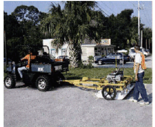
The 3-D underground imaging unit, which measures eight feet wide by three feet deep by 2 1/2 feet high, is pulled by a small all-terrain vehicle and can scan approximately one acre per day.
