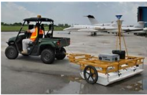
FIGURE 1 3D Radar system with dedicated tow vehicle
