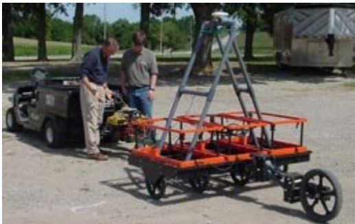
FIGURE 2 Multi-sensor EMI system with positioning hardware
