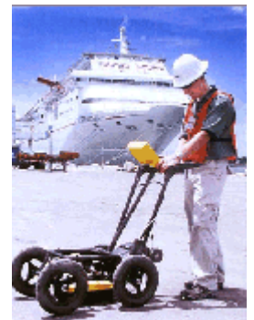
A typical digital GPR system consists of transmitting and receiving antenna elements, a central control unit and a field-ruggedized video display.
