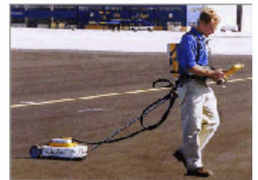
The prospect of an array of limitations presented at project sites requires that a GPR operator possess the maximum amount of information about that site prior to proceeding with a GPR investigation.
